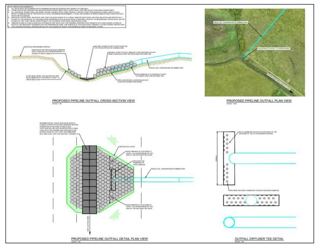
Figure 3.7 Outfall design. Source Dwg. No. 24821-MWP-00-00-DR-C-1003 (MWP) | not to scale
