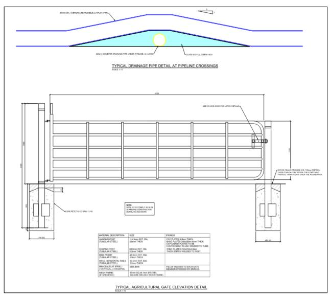
Figure 3.6 Agricultural gate design. Source Dwg. 24821-MWP-00-00-DR-C-0404 (MWP) | not to scale.
