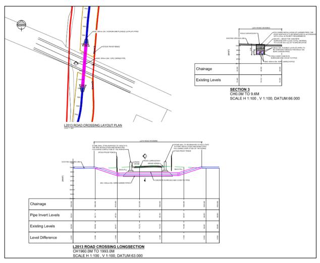
Figure 3.10 Proposed L2013 road crossing detail. Source Dwg. 24821-MWP-00-00-DR-C-0402 (MWP) | not to scale
