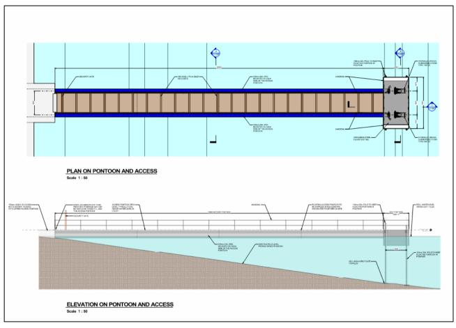
Figure 3.3 Configuration of the 2 pumps and floating pump pontoon. Source Dwg. 24821-MWP-00-00-DR-C-1004 (MWP) | not to scale
