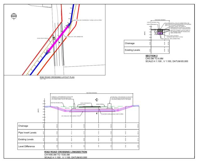
Figure 3.9 Proposed R362 road crossing detail. Source Dwg. 24821-MWP-00-00-DR-C-0401 (MWP) | not to scale
