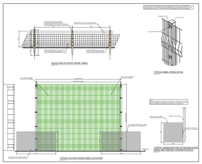
• The paladin fence posts will be secured to concrete blocks (Kelley Blocks or equivalent) so as to avoid disturbance of the underlying ground. Refer to the drawing in Figure 3.8 for details of fences.
