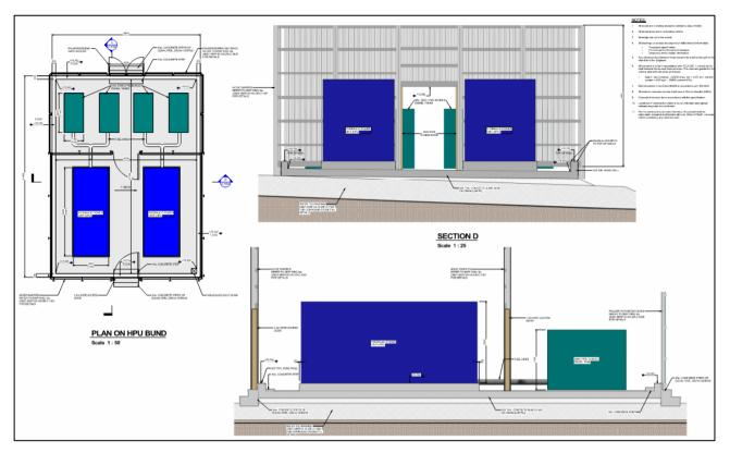
Figure 3.5 Configuration of concrete bund containing 4 no. fuel tanks and 2 no. HPUs. Source Dwg. 24821-MWP-00-00-DR-C-1006 (MWP) | not to scale
