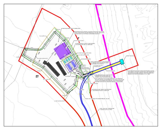
Figure 3.1 Proposed intake compound and pump layout. Source Dwg 24821-MWP-00-00-DR-C-1001 (MWP) | not to scale
