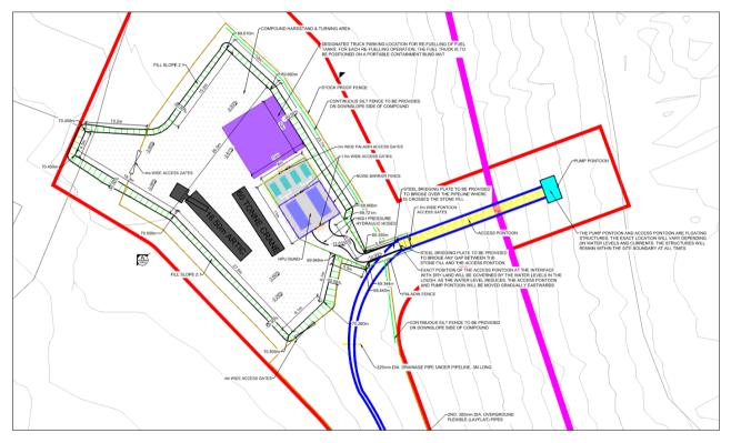
Figure 3.4 Intake compound, floating access pontoon and pump pontoon. Source Dwg. 24821-MWP-00-00-DR-C-1001 (MWP) | not to scale
