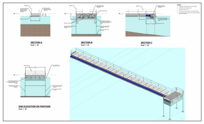
Figure 3.2 Design details of the pump pontoon (intake system). Source Dwg. 24821-MWP-00-00-DR-C-1005 (MWP) | not to scale
