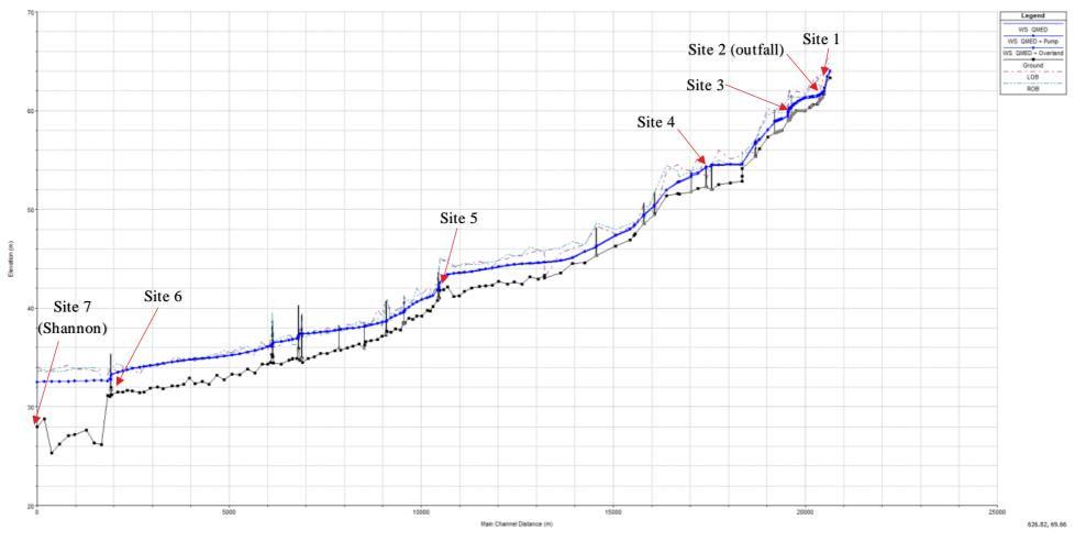
Figure 5.6 Longitudinal section of Cross River with Qmed and with pumped flows, proposed outfall location at 2050m distance (MWP, 2024)
